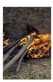
Figure 2: Firing bricks using wood as a fuel. Photo: Practical Action.
